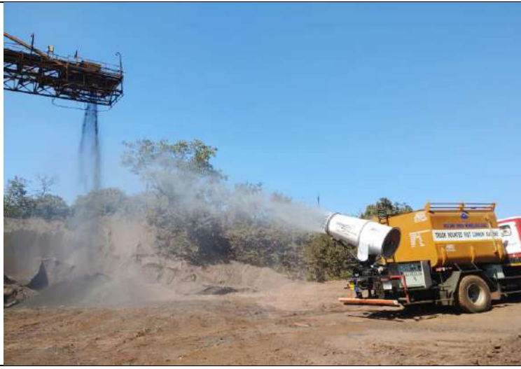
Truck Mounted Mist Canon Deployed at Near Fines Stacker
