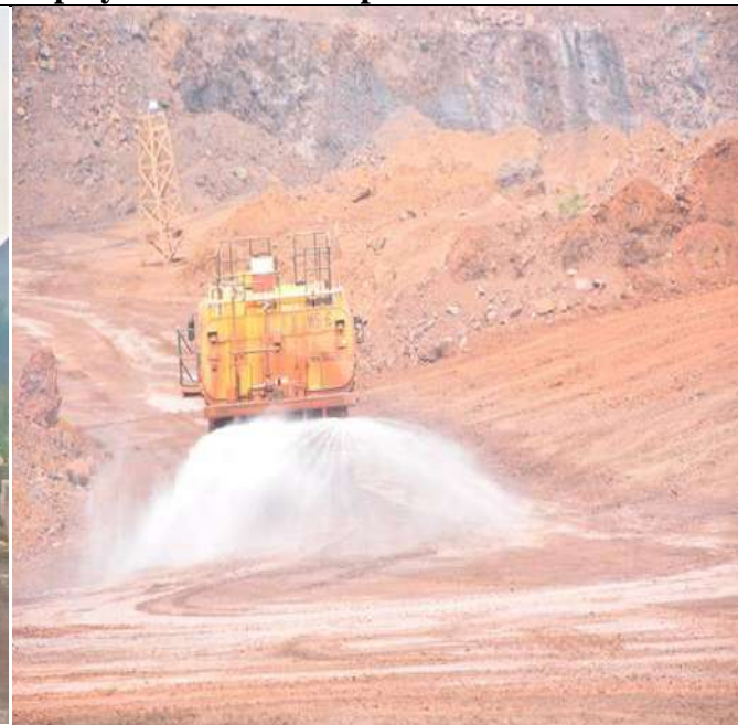
28 KL Mobile Water Sprinkler Deployed at F and G Area Haul Road
