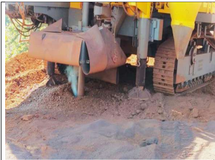
Drill Machine with Wet Drilling Facility Deployed at F and G-Area
