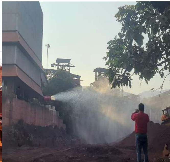
Rotating Fog Canon Installed at Lump Loading Plant
