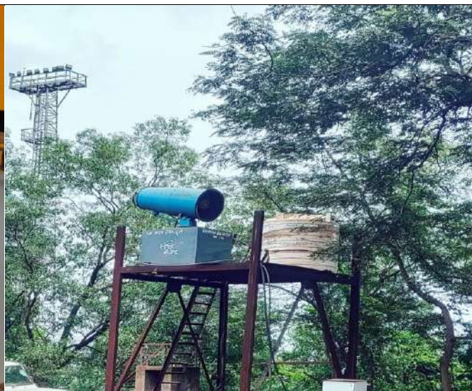
Rotating Fog Canon Installed at SSP
