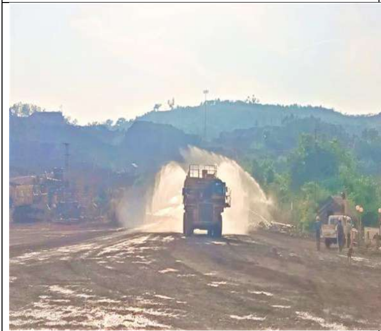
28 KL Mobile Water Sprinkler Deployed at F and G Area Haul Road
