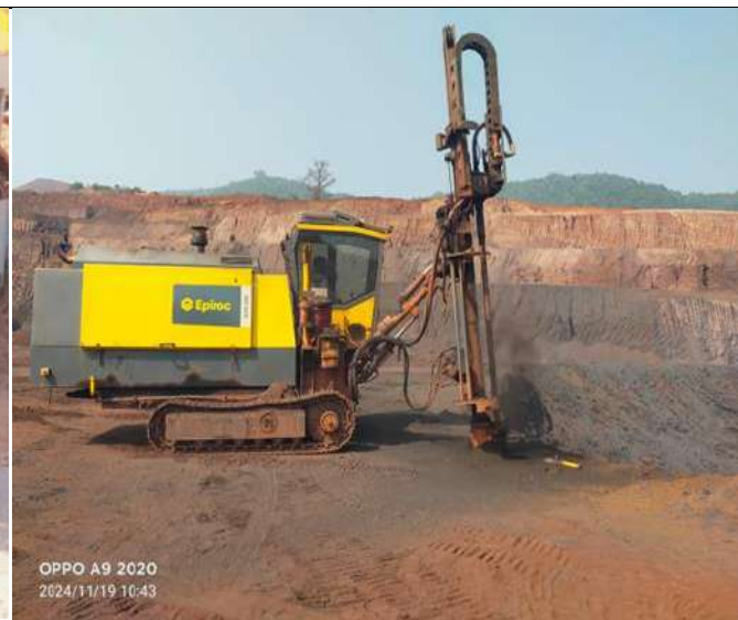
Drill Machine with Wet Drilling Facility Deployed at D and Panposh Area
