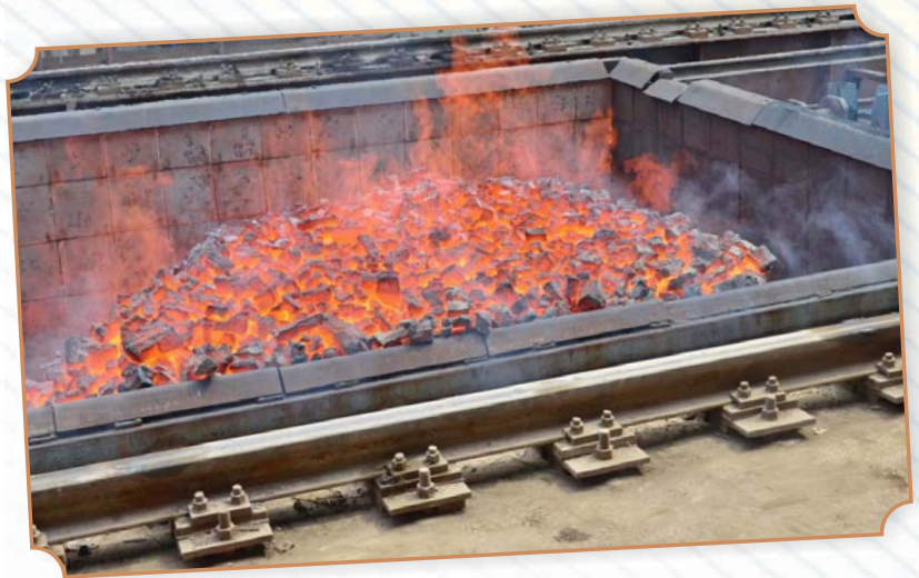
Hot coke obtained from RSP COB #6 after first oven pushing was commenced successfully
