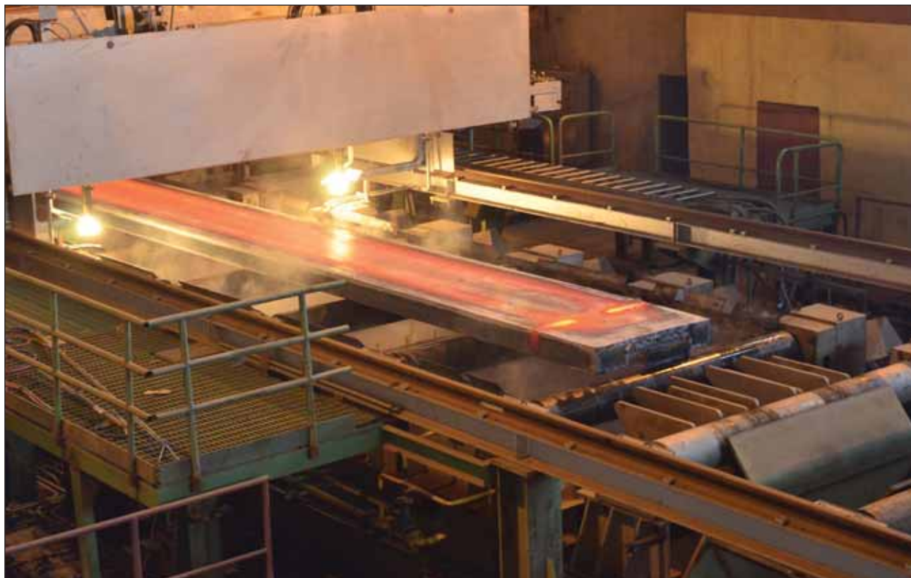
First batch of slabs being cast from the New Slab Caster at Rourkela Steel Plant.
